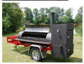
A Mobile Cooker / BBQ pit is virtually an oven on wheels. The cooking unit is mounted to the frame of the trailer unit.
